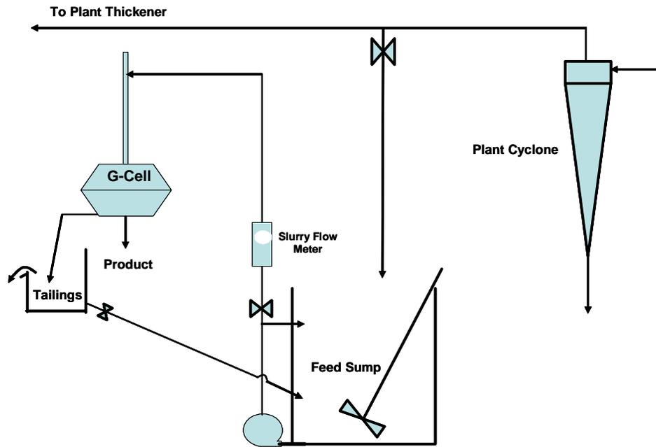
Figure 1: A schematic diagram of the experimental setup utilized for the G-Cell study conducted at a coal preparation plant site in the US
