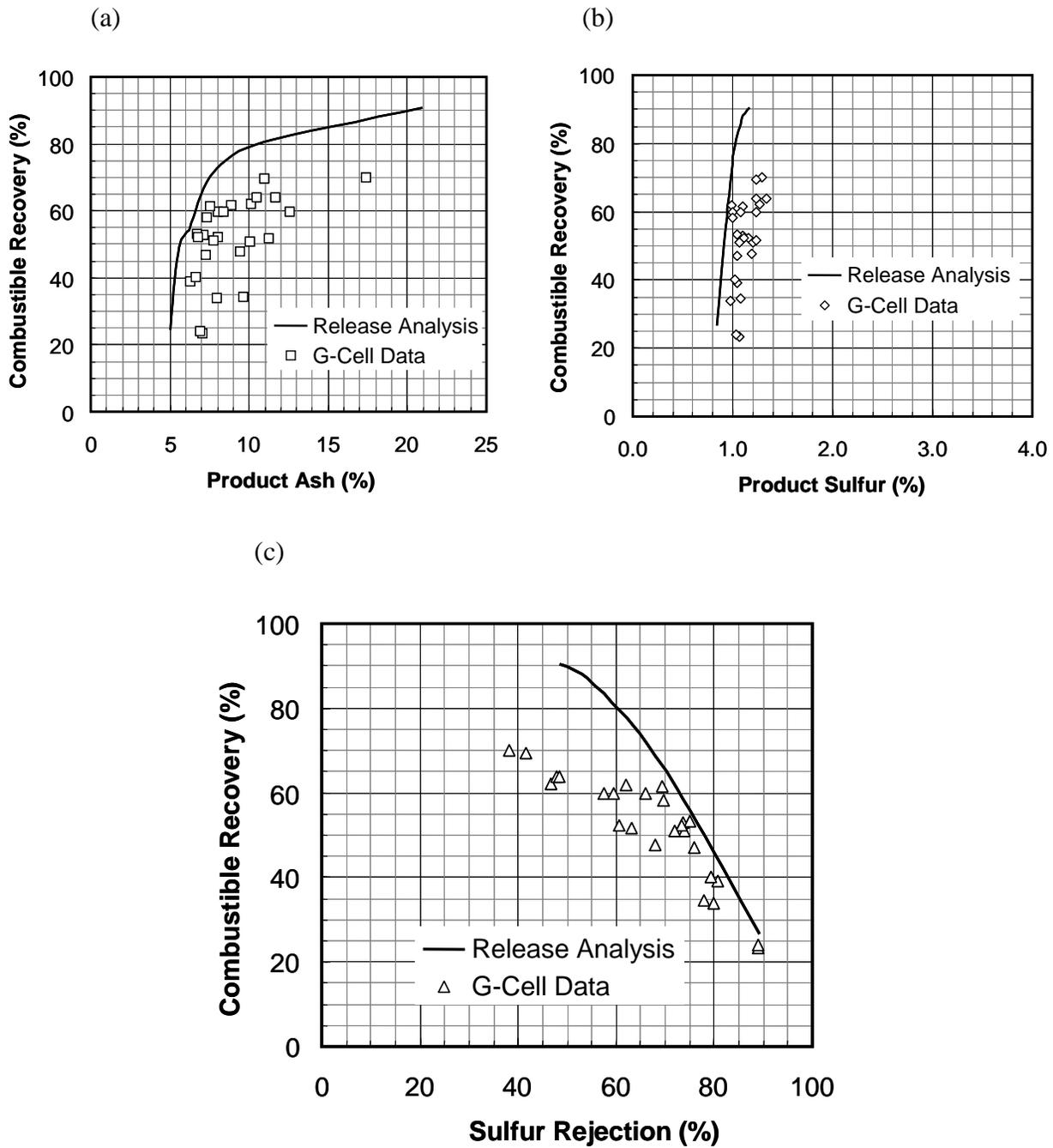
Figure 2: Metallurgical performance data obtained from G-Cell experiments in comparison the ideal flotation performance obtained from Release analysis
