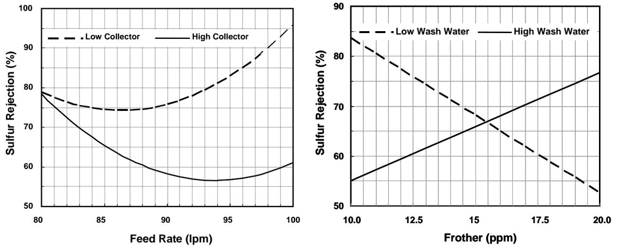
Figure 5: The parametric effects on sulfur rejection response
