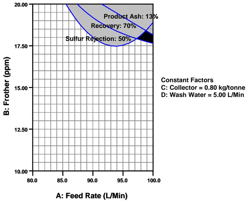
Figure 6: Optimized experimental conditions to achieve a desired separation performance, which is described as a combustible recovery of 70% or greater, sulfur rejection of 50% or greater and a product ash content of 13% or lower
