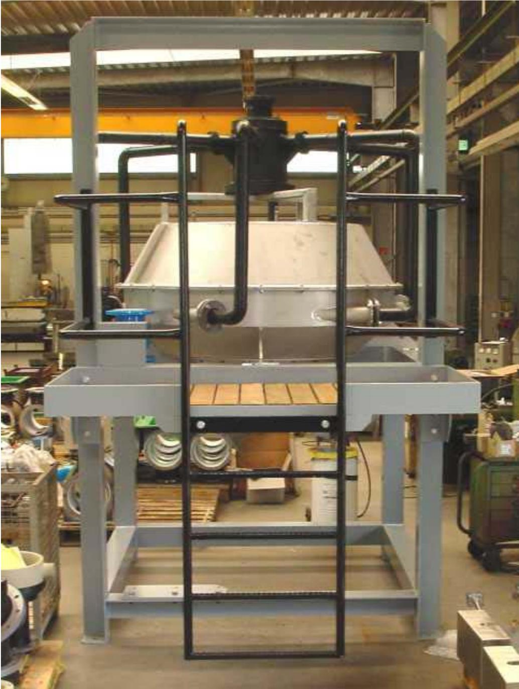
*Picture.3 Test rig Imhoflot G17 1,7 m diameter, feed rate 150 m<sup>3</sup>/h for potash cleaning*
