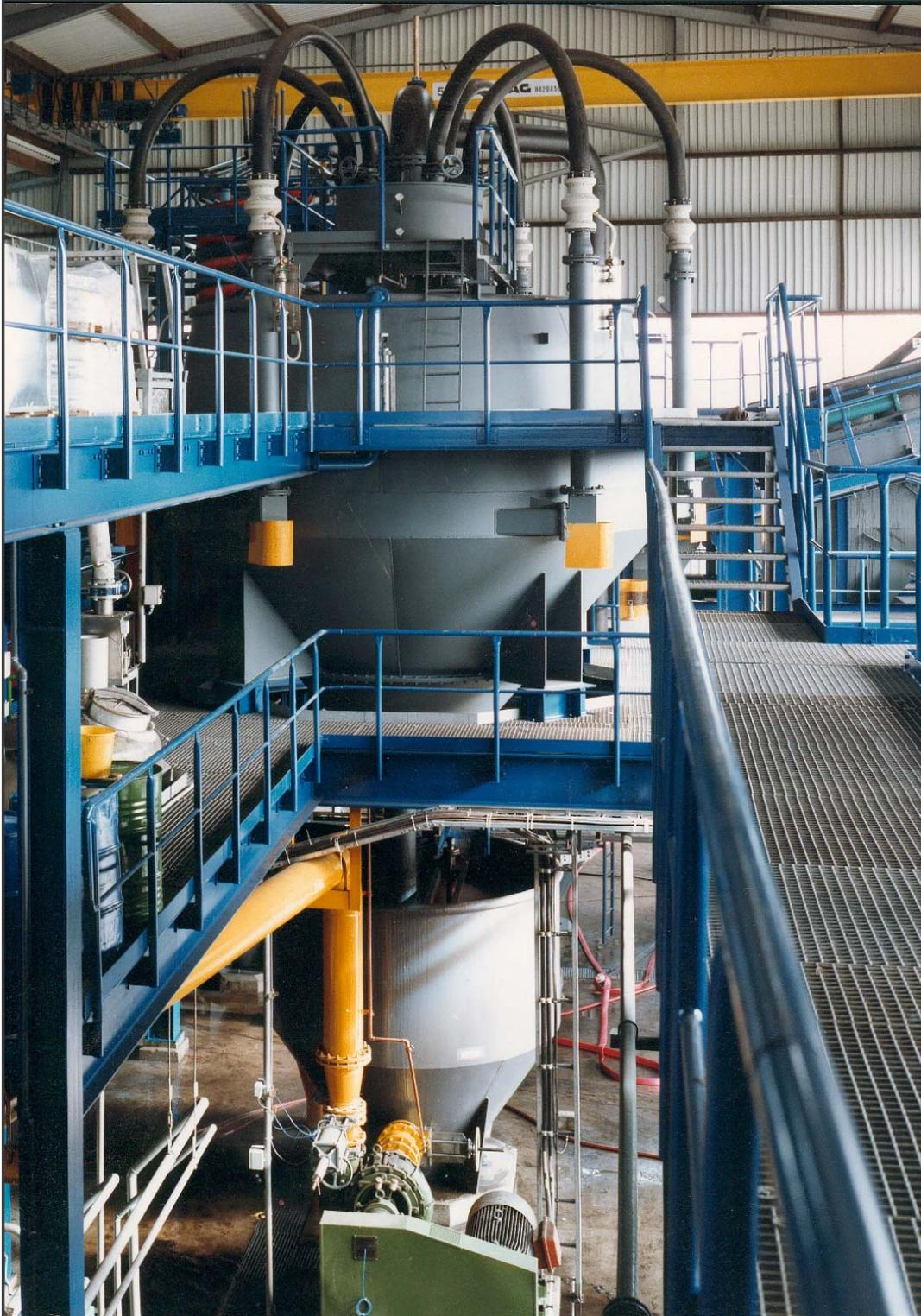
*Picture 1 First pneumatic cell 1988 in Germany, treating coal ponds*
